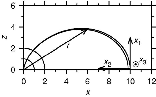
FIG. 1. Simulation domain in dipolar coordinates (upper half plane only shown) where  $x_3$  is positive increasing out of the page. The circle of radius 2 defines the “ionospheric” boundary in the present simulations. For comparison, the circle of radius 1 defines the Earth’s surface.  $\theta$  is the angle subtended from the  $z$  axis.
