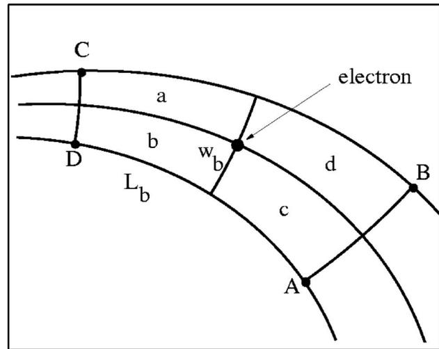
FIG. 10. Example of modified bilinear interpolation scheme in dipolar coordinates.  $L_b$  is the approximate length along  $x_1$  and  $w_b$  the approximate width in the  $x_2$  direction of subcell  $b$  (from Ref. 18).
