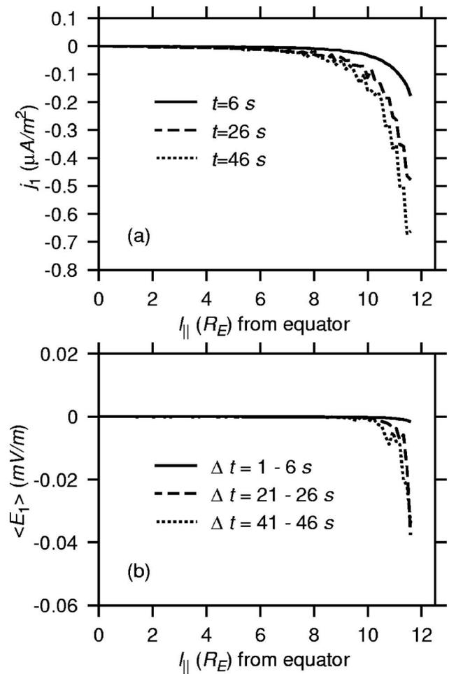
FIG. 9. (a) Parallel current density along  $x_2=0.1003$  as a function of distance along the field line (measured from the equator). (b) Same, but for time averaged parallel electric field (averaged over the 5 s intervals indicated).
