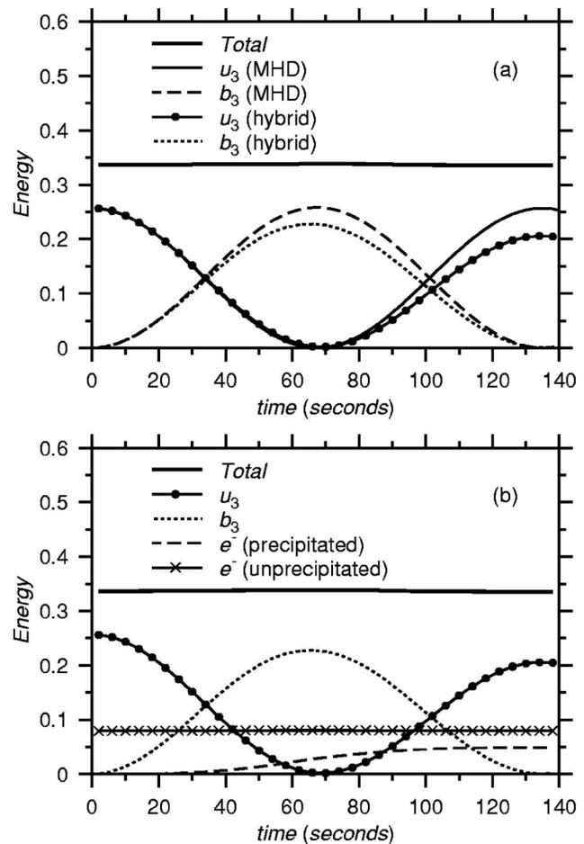
FIG. 7. (a) The energy in the azimuthal velocity,  $u_3$  and azimuthal magnetic field  $b_3$  from the hybrid model (as a function of time for half an Alfvén period) contrasted with the same from the cold plasma MHD model. (b) Total and component energies for the hybrid model.
