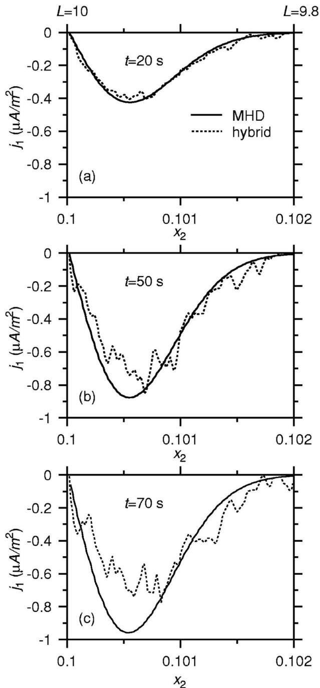
FIG. 3. Parallel current density at the northern ionospheric boundary at  $t=20$  s (a),  $t=50$  s (b), and  $t=70$  s (c).
